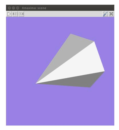
By holding down the left button of the mouse while it is moved on the graphics window, the camera can be rotated showing different views of the pyramid. The two plot options [scene\_elevation], page 944 and [scene\_azimuth], page 944 can also be used to change the initial orientation of the viewing camera. The camera can be moved by holding the middle mouse button while moving it and holding the right-side mouse button while moving it up or down will zoom in or out.
